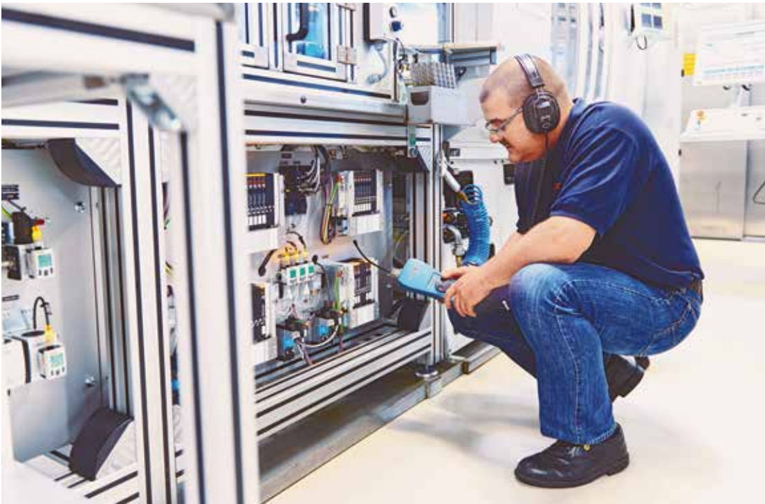
Bernard Kohl uses a leakage-detection device to determine the cause of the increase in compressed air consumption
